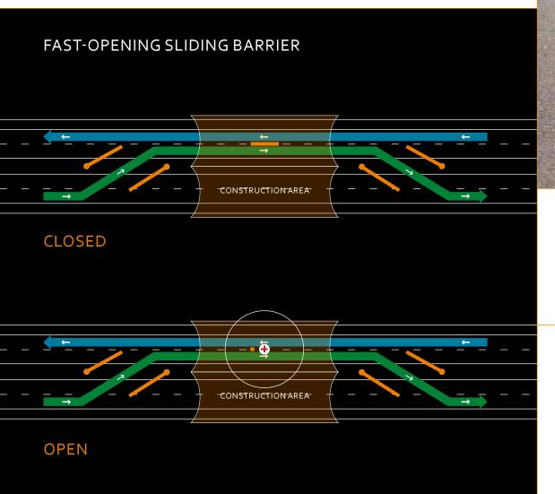
The sliding barrier opens the way between the two lanes.
